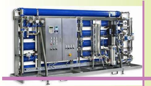
Reverse osmosis is a membrane - Technology filtration methos that removes many types of large molecules and ions from solutions by applying pressure to the solution when it is on one side of a selective membrane, it is a process of physical separation of dissolved solids and minerals present in water. This technology uses the principle of osmosis, wherein the mineral concentration of raw water is redced by applying high pressure through a semi permeable membrane.
